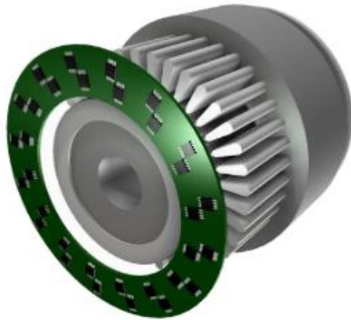
Fig. 1. Set-up of ISCAD: the aluminium bars inside the stator core are connected to a short circuit ring on the backside. A dedicated power electronics unit is connected to each aluminium bar.
