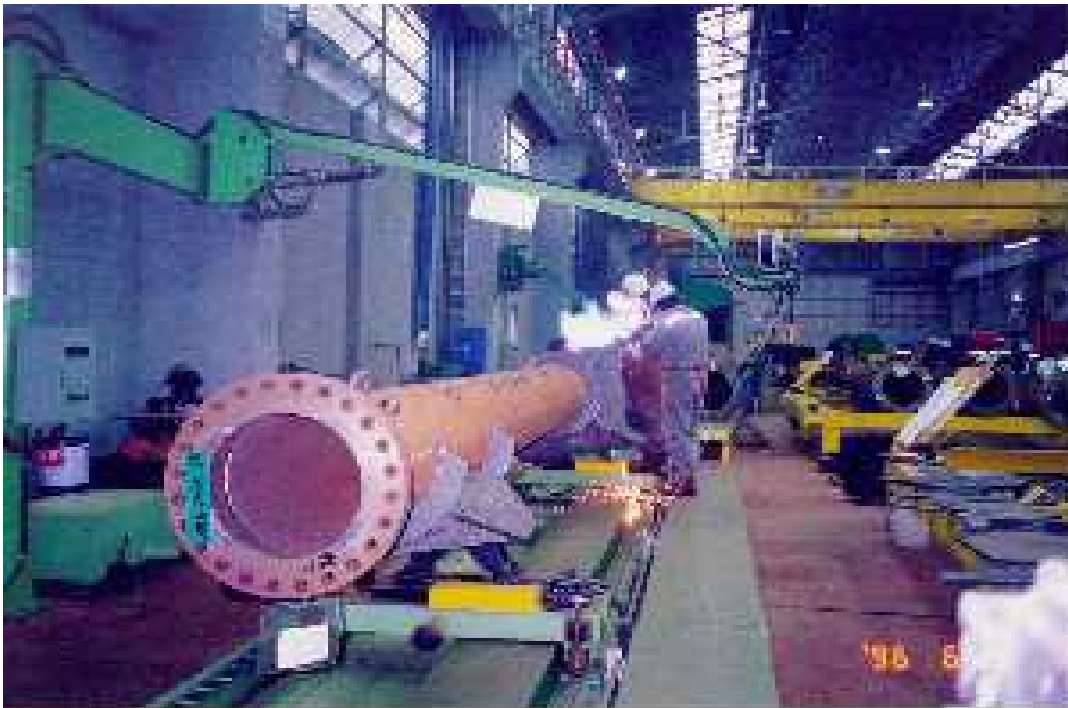
Manufacturing of 765 kV tubular tower
